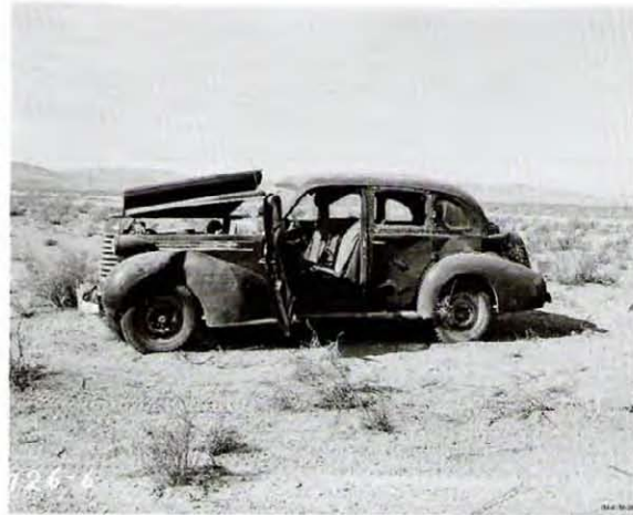
Oldsmobile four-door sedan placed at one mile from ground zero, oriented at about a 45-degree angle to the blast. The windows on the blast side were broken. One was blown in and the other badly crushed. The windshield was cracked. The paint and tires on the blast side were charred, but the tires remained inflated. The side facing the blast was bashed in. The hood was lifted but not blown off. Apparently the door on the blast side had been left open, because there was a sharp line of demarcation of charred area visible on the upholstery. The motor seemed undamaged, as was the battery, given that the horn still operated. Source: Los Alamos National Laboratory.
